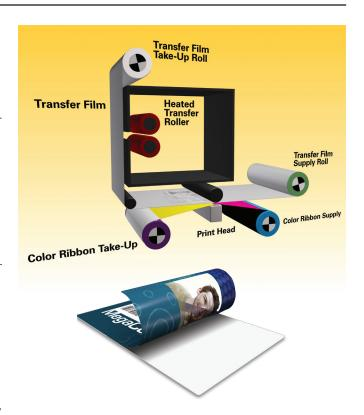
Zebra's patented image transfer process applies film to both sides of the card in a single pass, drastically reducing the print time.
